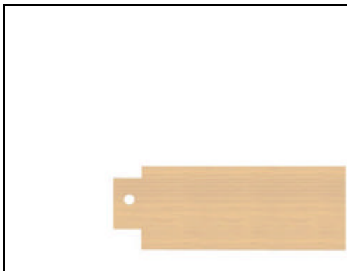
b. New timber splice, with replacement tenon.
